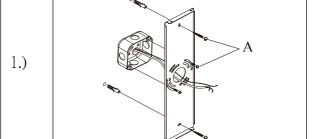
Step.1: Install Mounting bracket(A) to outlet box.
