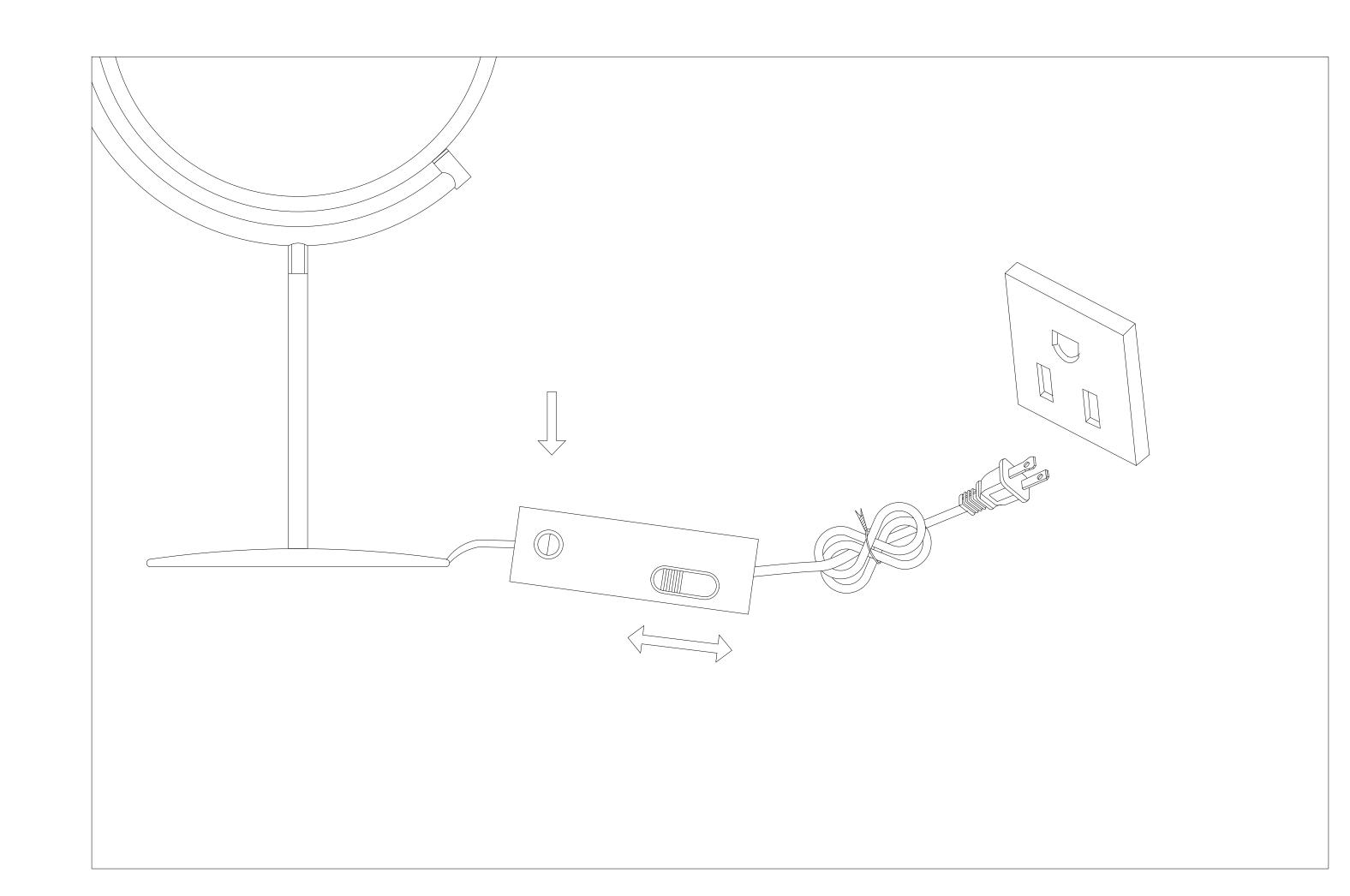
Step1 :pressed the switch to turn on light
